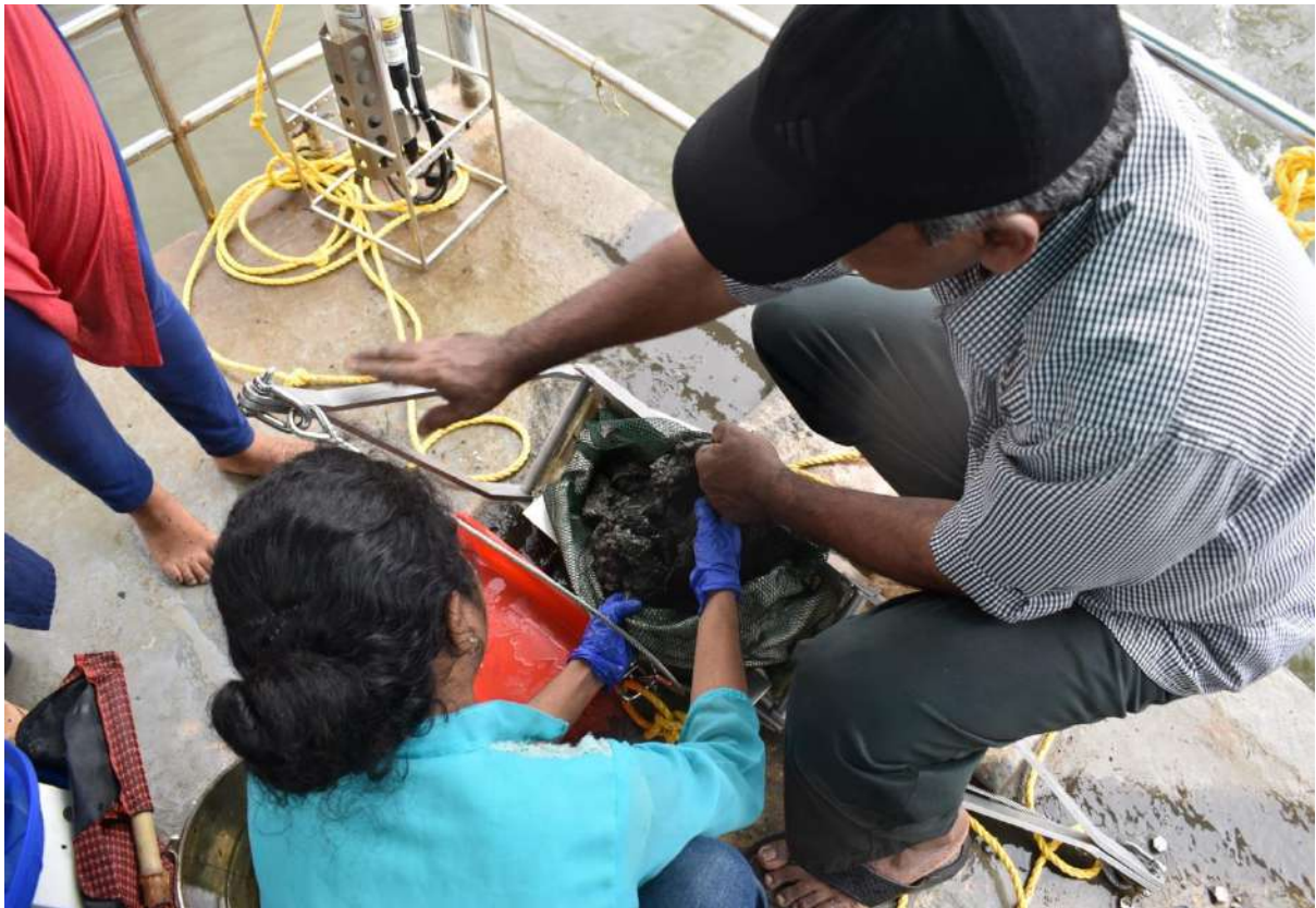
Figure 6 B:Collection of Sediment Grab Samples from South Sector of Vembanad Lake.
