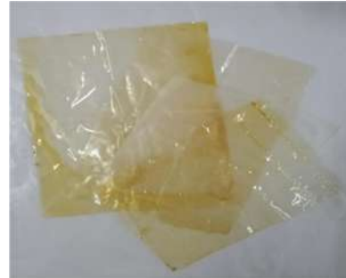
Films prepared with semi refined carrageenan from Gracilaria crassa and Gracilaria edulis with chitosan
