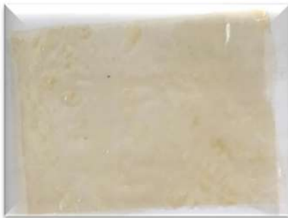
Films prepared with semi refined carrageenan from Gracilaria crassa and Gracilaria edulis with chitosan
